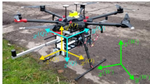
**Figure 2.** DJI M600 drone and sensor rig mounted to it. The weight of the payload is just below 5 kg. The axes with superscript (O) refer to the Ouster (sensor) reference frame, the ones with (Q) refer to the Quanta frame, and finally, those with (W) refer to the world frame, where  $x^{(W)}$  points east and  $y^{(W)}$  north.
