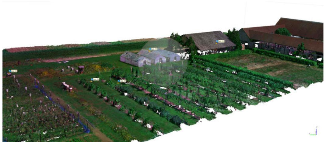
**Figure 14.** The resulting multispectral point cloud from the Bottelare dataset, here colored using the bands corresponding with the red, green, and blue wavelengths.
